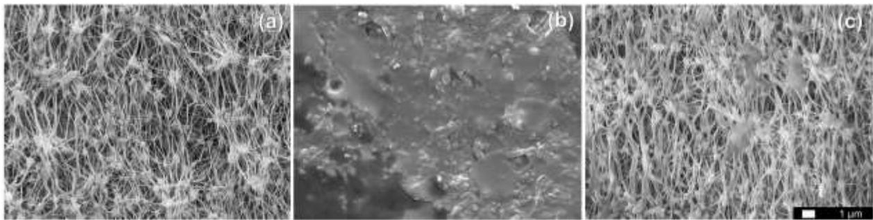
**Figure 4:** Scanning electron microscopy images for the (a) unused membrane, (b) feed-side of the membrane after the experiment, and (c) distillate-side of the membrane after the experiment, for the 100-day experiment.
