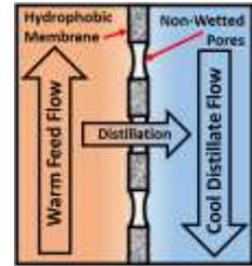
**Figure 1:** Membrane distillation diagram.
