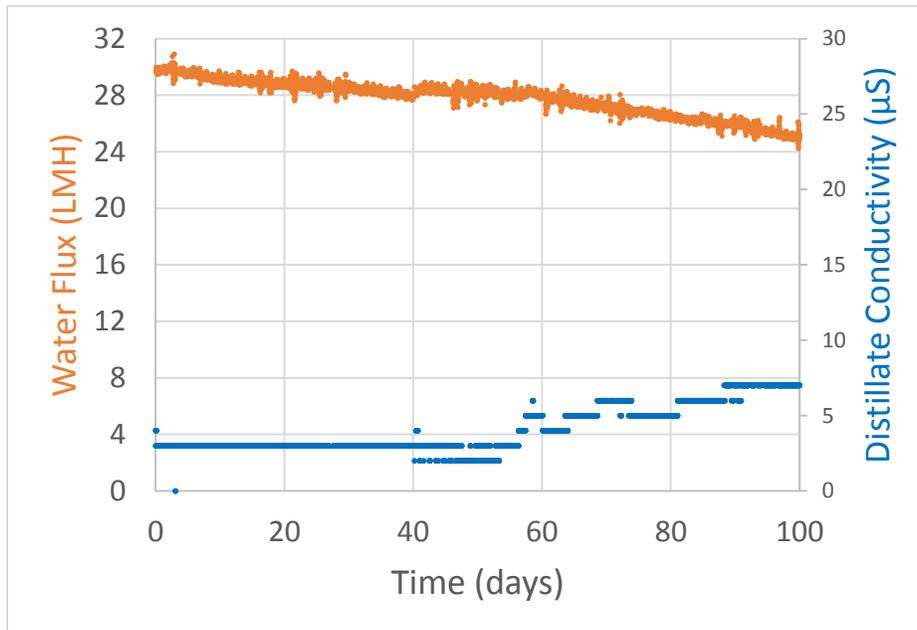
**Figure 2:** Water flux and distillate conductivity over time for 65 °C feed with 35 g/L NaCl and 38 °C distillate.
