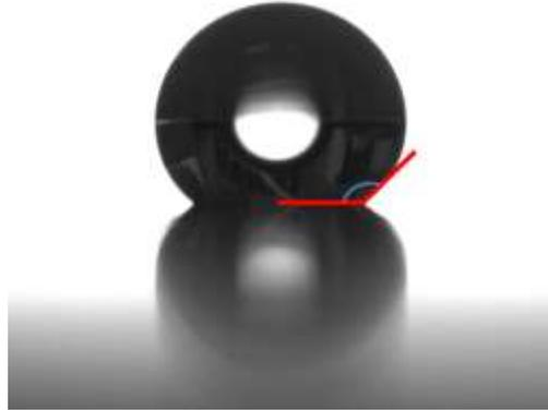
**Figure 3:** A goniometer image used to measure the contact angle of a drop of water on the membrane surface.
