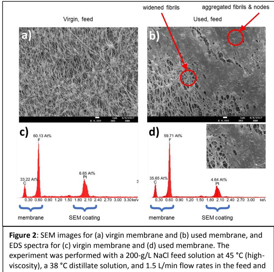
**Figure 2:** SEM images for (a) virgin membrane and (b) used membrane, and EDS spectra for (c) virgin membrane and (d) used membrane. The experiment was performed with a 200-g/L NaCl feed solution at 45 °C (high-viscosity), a 38 °C distillate solution, and 1.5 L/min flow rates in the feed and
