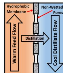
**Figure 1:** Membrane distillation diagram.
